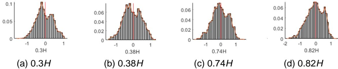
Fig. 2 Observed bimodal PDF at corner of front wall of principal building
